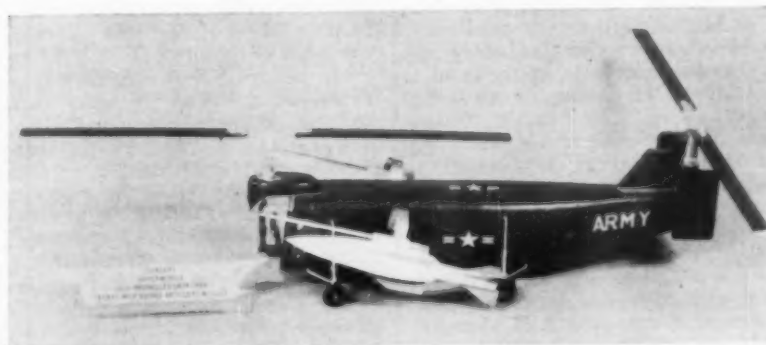
LAUNCHER for 20-in. guided artillery missile is suspended on side of HSL-1 model.
